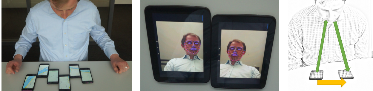
Figure 1: Left: HeadPhones allows dynamic registration between mobile devices using the human head as reference frame. Middle: Head pose estimation and concatenation is used to determine the relative positions of the devices to each other. Right: Transformation between two devices is computed by chaining the (inverse) transformations between each device and the user's head.
